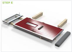
Confirm the position and orientation of the toplight before installing any fixings.
