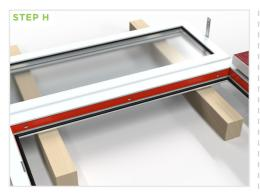
Drill 3 no. x 4.5mm diameter pilot holes through the head of the doorset frame and up into the toplight frame. Pilot holes should be located between 150mm and 200mm from corner of frame and at the mid point (just off centre) so you have 3 in total.
