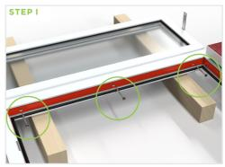
Ensure the screwdriver is set to a low torque and slowly do up the 3 no. 4.8 x 90mm long countersunk screws. The head of the screw should finish slightly below the surface of the intumescent seal.
