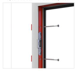
and of the correct thickness as to not cause the frame to bow when the fixings are installed.
