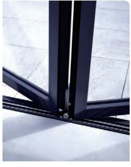
A unique, pivoting axle in the rollers allows the wheels to follow any undulations in the stainless-steel tracks underneath. Combined with sealed bearings in the stainless-steel wheels and lateral rollers, the doors will glide effortlessly and smoothly for years to come.
