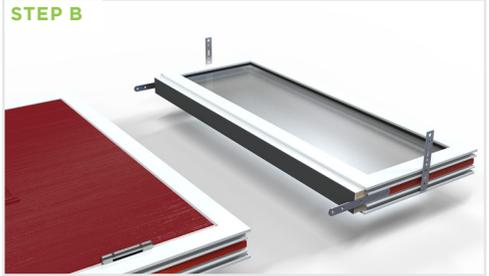
Screw (minimum size 4.3 x 40mm) fix 1 x VEKA steel frame strap to both vertical parts of the top light frame. They should be positioned approximately centrally along the length.
