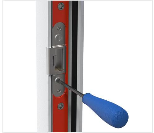
Checks should be made to ensure the lock hooks are engaging the keeps in a **central position** to ensure reliable operation of the lock throughout ongoing life service.
