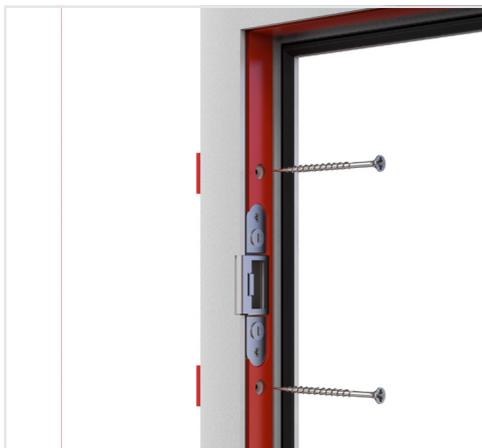
and of the correct thickness as to not cause the frame to bow when the fixings are installed.
