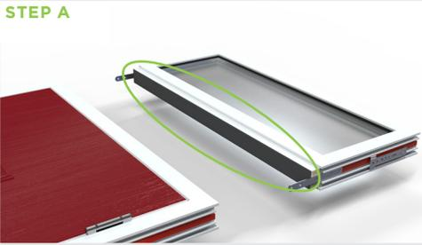
Inspect the coupler of the top light that is factory fixed to the top light frame. Confirm the grey intumescent 1mm thick pad that is applied to the coupler face where it will join to the doorset frame is not damaged. If it is damaged - do not proceed and contact Door-Stop for replacement.
