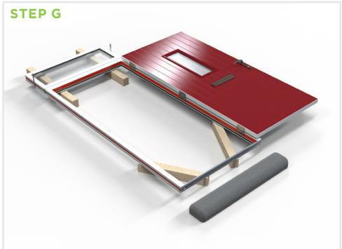
Once the 4 no. 4.3 x 40mm screws are in place, carefully open the door and lay it gently on the protected bearers.
