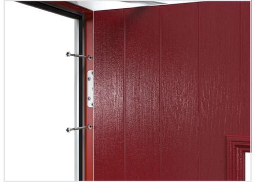
The pilot hole for the fixing should be countersunk to ensure the head of the fixing is slightly below the surface of the intumescent seal. Care should be taken not to over-tighten fixings. It is acceptable for the wall fixing to be positioned through the intumescent seal.
