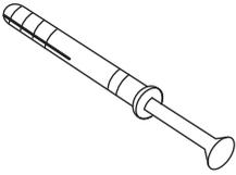
Fixings are required that are suitable for the specific wall type construction the doorset is being secured into. The fixings must allow a minimum 45mm penetration into the wall structure, excluding the door frame and gap between the frame and the wall. The fixing should be of a minimum size of 4.8mm diameter countersunk fixing.
