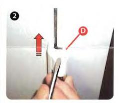
Carefully remove the top cap and with a 6mm socket spanner rotate the hex pin (D).
